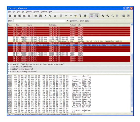
The capture is continuing to write packets to the output file. If we ping r2 from r1, then hit the "reload this capture file" icon we see:
